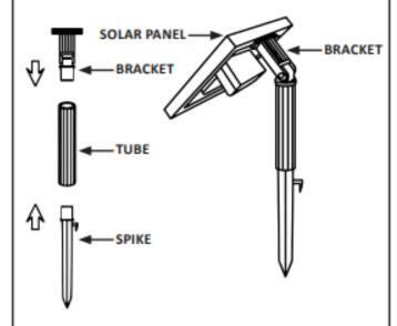
**5.** Insert the spike into the ground. Position the solar panel to face south (in the northern hemisphere) to make the most of daylight hours. It is important to angle the solar panel towards the sun when the sun is at its highest point. Ensure trees, shrubs, or buildings do not shade the solar panel.
