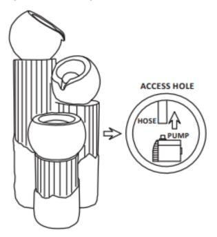
Extend the pump and LED light cables through the access hole in the back of the fountain, cables are ready for connection to the solar panel.
