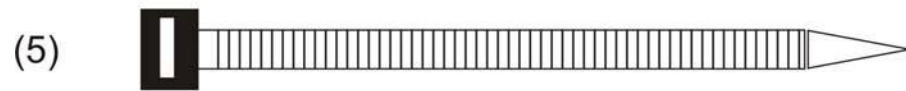
(5) Collgation To bind the PVC tube with the pump. Ensure that link up tight.
